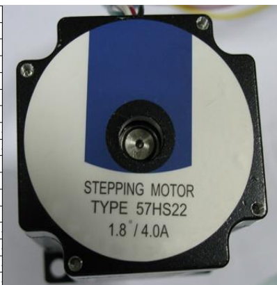
Motor nameplate/ stepper angle=1.8°
